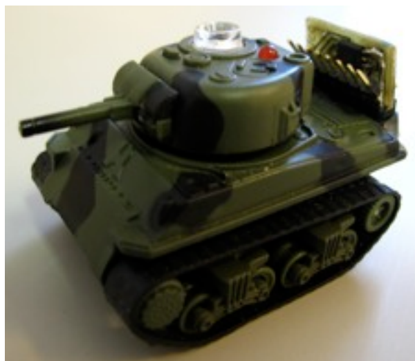
The modified Robot Soccer Tank, with custom micro-controller board
