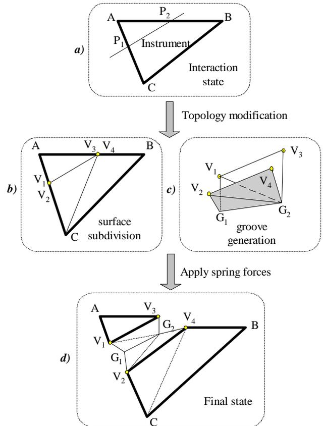
**Figure 6: Surface subdivision and groove generation for midway triangles**
